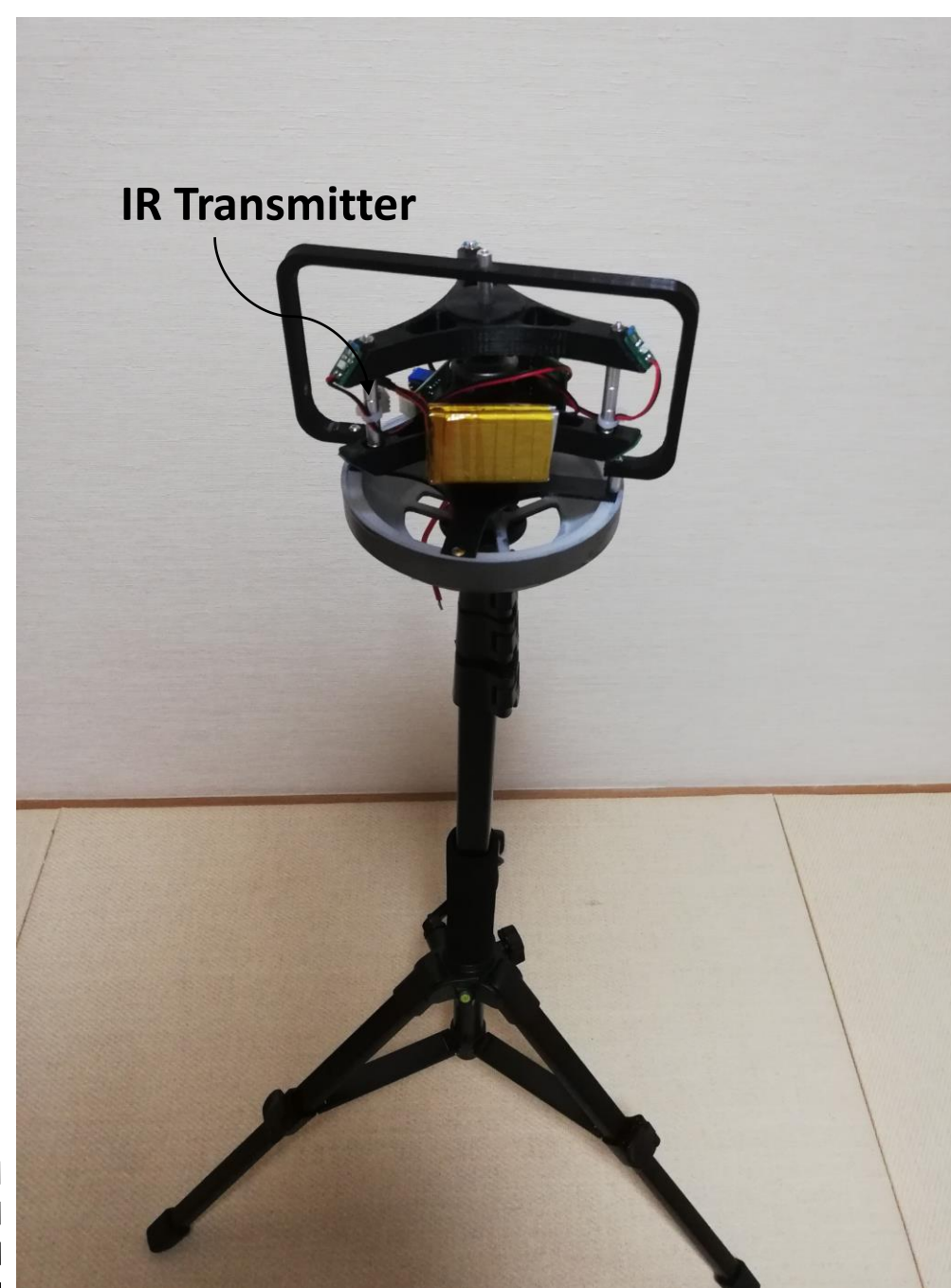
IR Transmitter Station
