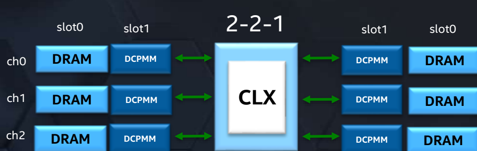
Sample Cascade Lake (CLX) Platinum/Gold Socket with Apache Pass (DCPMM)
